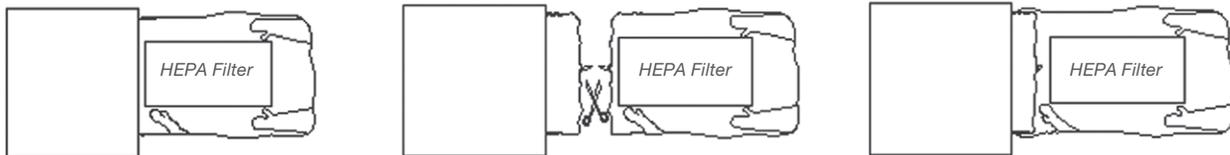
3. Remove bag stub using bag stub removal glove sleeve of the new bag. Draw stub into sleeve by turning sleeve inside out. Install new filter using glove sleeves. Seal and detach bag stub/glove sleeve. Fold new bag inside bagging ring and replace access door.
