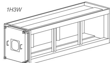
Note: All housings are available with optional prefilter sections behind primary filter door or with a separate prefilter door.
