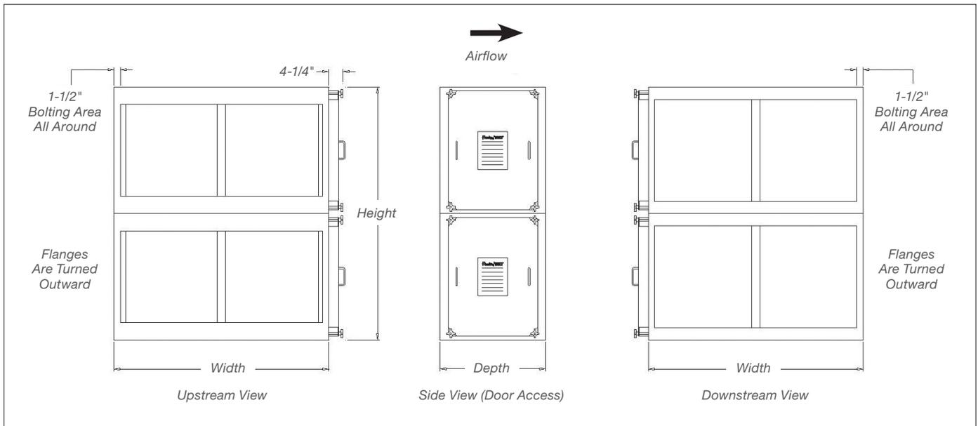
The D/6 in this model number represents the following model numbers: **BG1-1H1W-CCD-304-D1** to contain a HEPA filter, or **BG1-1H1W-CC6-304-D1** to contain a Carbon Adsorber.
