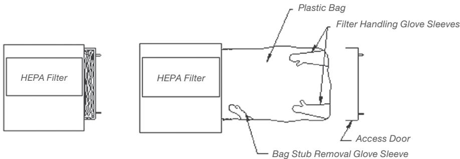
2. Carefully draw contaminated filter into bag and place filter (in bag) on stand or table. Remove arms from bag. Seal bag between access port and filter. Cut bag, leaving bag stub attached to access port. Place new filter into a new bag. Place new bag over bag stub attached to access port.
